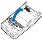
3 Insert the SIM card into the holder as shown, beveled corner first, with the gold colored contacts on the SIM card face up (away from the phone).
